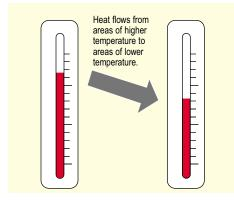
2. The greater the difference in temperature between two adjacent areas, the higher the rate of heat transfer between them.
